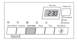
If this additional function is selected, the anticrease phase at the end of the drying cycle is lengthened by 60 minutes. The laundry can be removed at any time during the anticrease phase.
